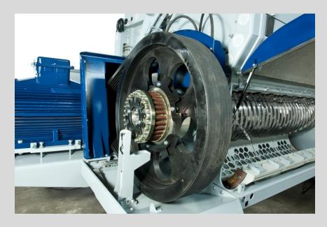
Protection against damage of machine caused by foreign objects.
